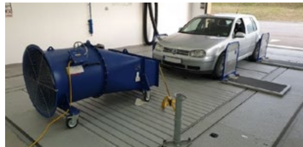
Fig. 3. Tested vehicle on chassis dynamometer
