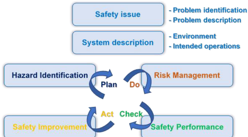
Fig. 1. Generic safety assessment process
